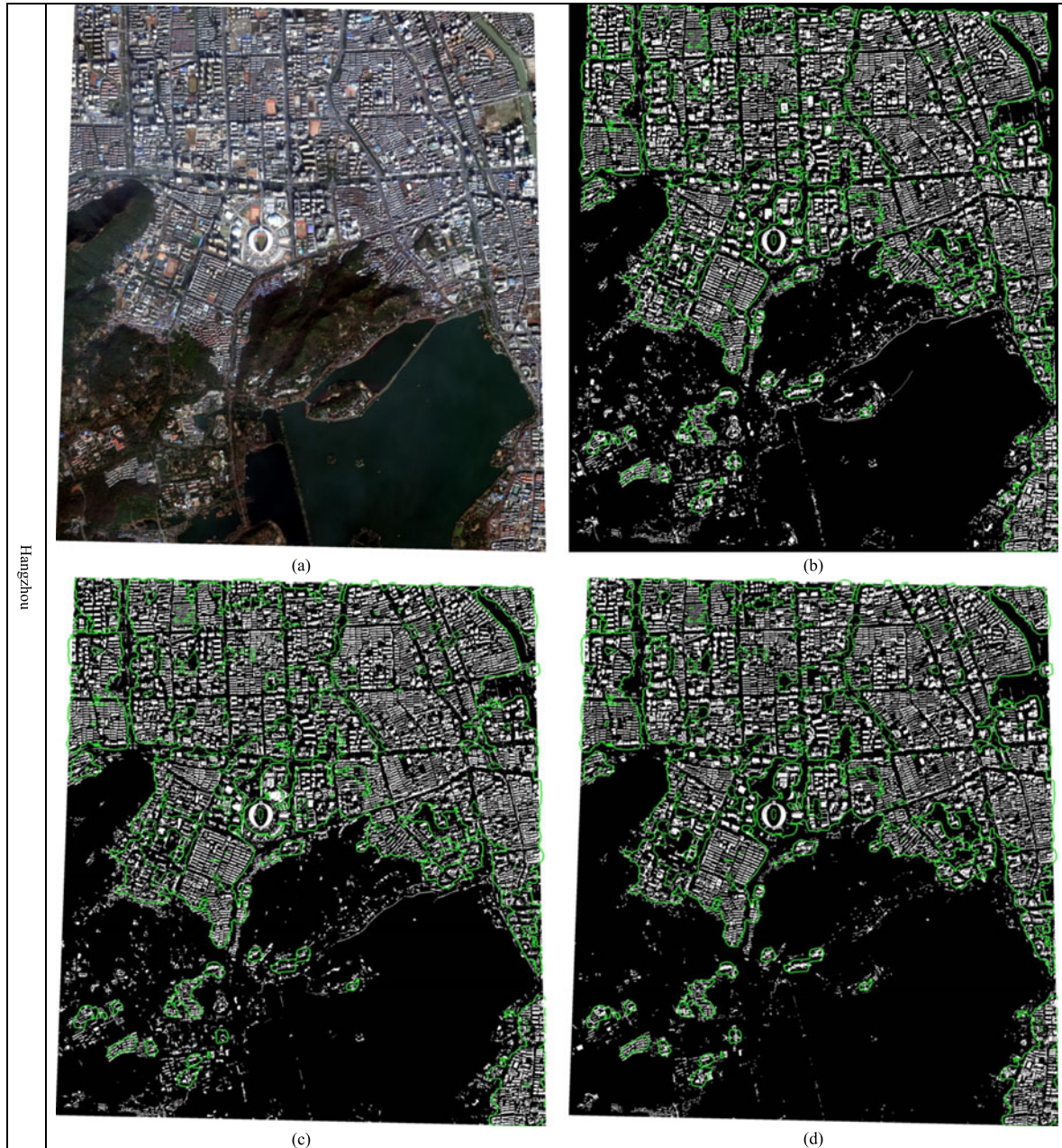
Fig. 7. Building detection results: (a) original RGB images; (b) building maps with the result of the MBI; (c) building maps with the result of DMP-SVM; and (d) building maps with the result of the proposed framework. The green color represents the boundary between the high-density and low-density areas.
