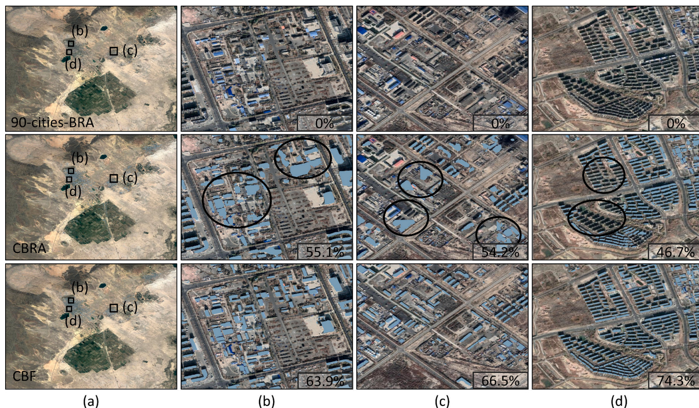
Fig. 19. Comparison of different products in Karamay. The first, second, and third row present the results of 90-cities-BRA, CBRA, and our CBF, respectively. Column (a) provides an overview of Karamay, with (b), (c), and (d) showing enlarged views of the black-boxed regions. The numerical values in the bottom right corner indicate the IoU of the current predicted result.
