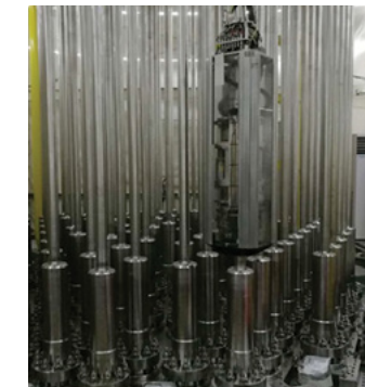
FIGURE 1. Ultrasonic inspection equipment for control rod. Credit: Xiaohong Li, Jun Zhang
