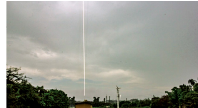
FIGURE 1. Testing of an artificial lightning strike on transmission lines.
