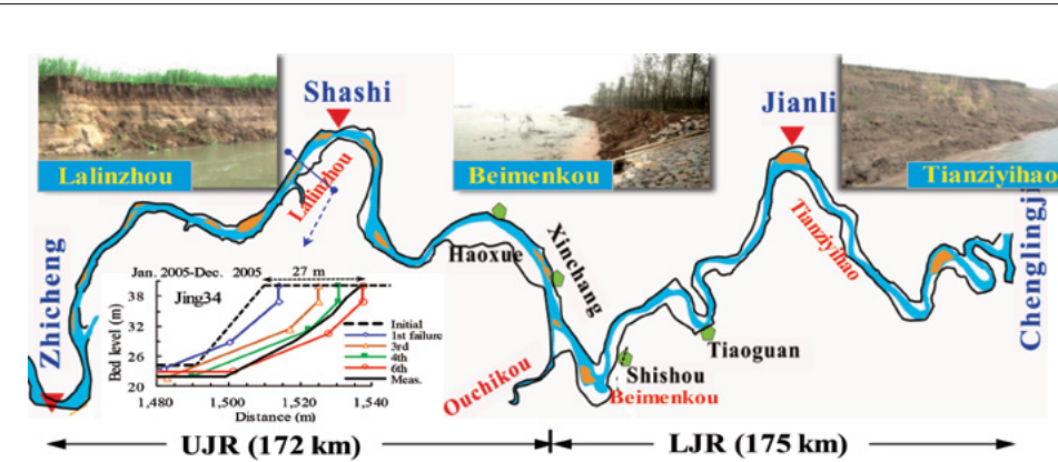
FIGURE 4. Changes in bank erosion along the Jingjiang Reach of the Middle Yangtze River after the Three Gorges Project began operation. UJR, Upper Jinjiang Reach; LJR, Lower Jinjiang Reach. Credit: Junqiang Xia
